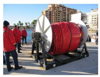
The Lamor Electric operated Storage Reel Heavy Construction model ESR H1722 is designed to store up to 200 m length of up to 2000 mm height heavy duty oil booms like Lamor HDB offshore rubber booms. The maximum storage capacity for each size and type of boom must be confirmed with Lamor representative.
