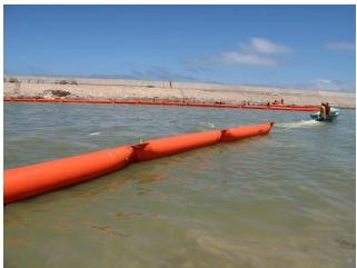
The Inflatable Light Oil Boom is a lightweight and durable air inflated boom that covers the increasing demand for harbors, nearshore and offshore oil containment boom configurations, mainly deployed for emergency oil spills and protection.
