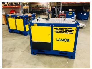
The Hydraulic Power Pack LPP 35 is used as a power source for skimmers and other hydraulically operated equipment such as boom reels, pumps etc. Equipped with a direct outtake, the LPP 35 can power multiple pieces of equipment simultaneously (for example a skimmer and an oil transfer pump) through a control stand or from an onboard optional control valve.
