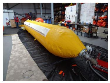
The LFT 10 is a durable floating storage tank designed for the storage of recovered oil primarily at sea but can also be used on land.
