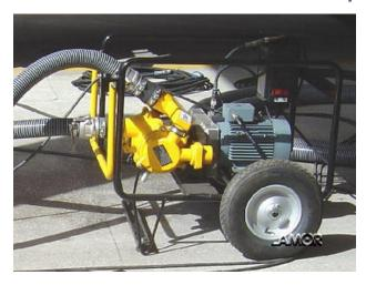
The Lamor LPP 7.5E is a small electric power pack with C 75 oil transfer pump built in the same frame. Optionally it can be equipped with ExProof additions for use in hazardous areas.
