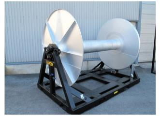
The Lamor Hydraulic operated Storage Winder HSR L1717 is designed to store up to 200 m length of 350-750 mm high foam filled oil boom (FOB), 150 m FOB 900 or higher, or 250 m inflatable light oil boom (ILB) or self inflatable Auto boom (LAB). The maximum storage capacity for each size and type of boom must be confirmed with Lamorrepresentative.
