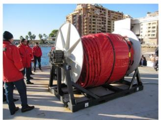
The Lamor Electric operated Storage Reel Heavy Construction model ESR H1722 is designed to store up to 200 m length of up to 2000 mm height heavy duty oil booms like Lamor HDB offshore rubber booms. The maximum storage capacity for each size and type of boom must be confirmed with Lamor representative.
