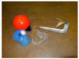
The Anchoring Set is a boom anchoring kit for smaller sized foam float and inflatable booms comprising of one 10 kg galvanized Bruce type anchor, 5 m of 10 mm anchor chain with 2 pcs shackle M12/Y, one 40 cm diameter anchor buoy and 50 m of 16 mm tripping line.
